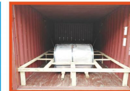
Coils Fixed In Container
