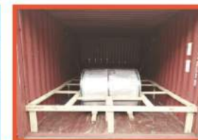
Coils Fixed In Container
